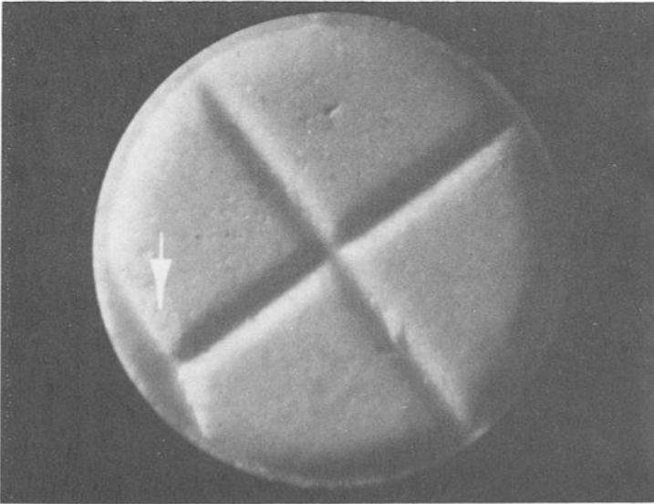
FIG. 1—Amphetamine sulfate "mini-bennie" showing gouge at edge and tiny lumps in groove bottoms. ( \times 10 ).
